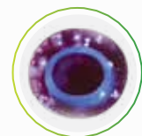
Cross section illustrating micro bubbles and smooth internal lumen
